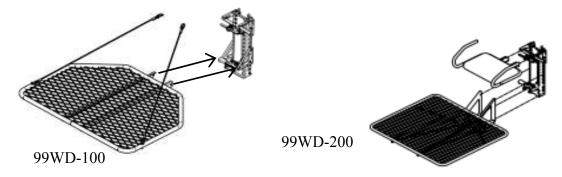
Attach the platform cables at the top of the elevator on the 99WD-100. There are no suspension cables for the 99WD-200 model.
