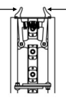
Push toward the inside with the thumb and index finger to lock the rail
