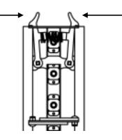
Push toward the inside with the thumb and index finger to unlock the rail
